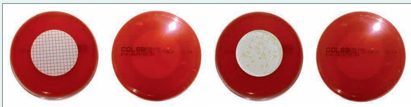
Fig. 4: Columbia agar plate with filter placed over it, above left: the front with filter placed over it and still without growth; above right: the back; below left: evidence of colony forming units (cfus) on the filter; below right: the back
