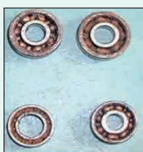
Figs. 3 to 5: Surface discoloration due to unsuitable detergents or water quality
