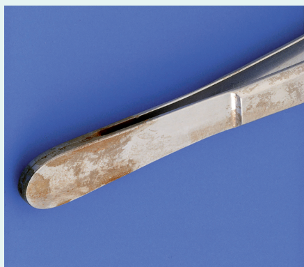
Fig. 3: Example of a surface change with crevice corrosion, surface corrosion
