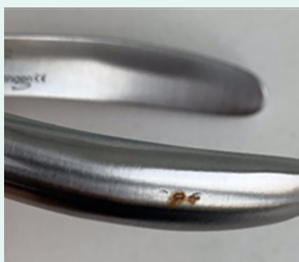
Fig. 6: Corrosion or residue
