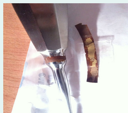
Fig. 8: Residues/corrosion below the marking tape - device should not be used
