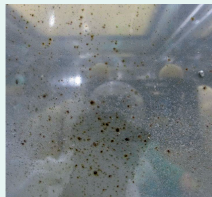
Fig. 10: Corrosion of WD rear chamber wall
