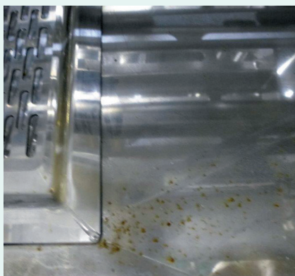
Fig. 9: Corrosion of WD chamber bottom
