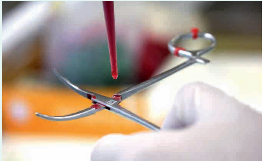
Figure 1: As defined TEST OBJECT , a Crile arterial clamp is used as per the guideline
